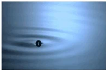
Walking arises as \gamma approaches the Faraday threshold \gamma_F
